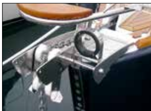
Bow bracket integrated with bow anchor fitting.
